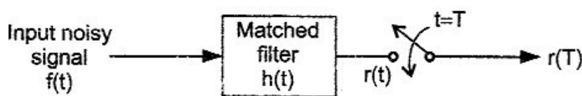
Fig. 4.8.2 Block diagram of a matched filter receiver
