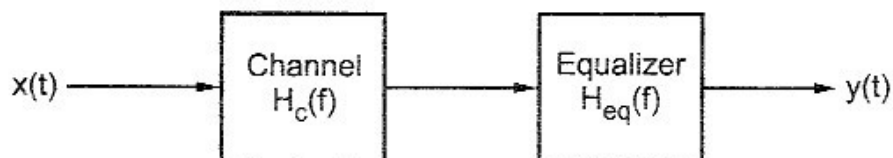
Fig. 4.13.1 Equalizer for correction of distortion introduced in the channel
